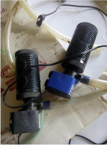
Figure 7: Water Filter cum Pump
