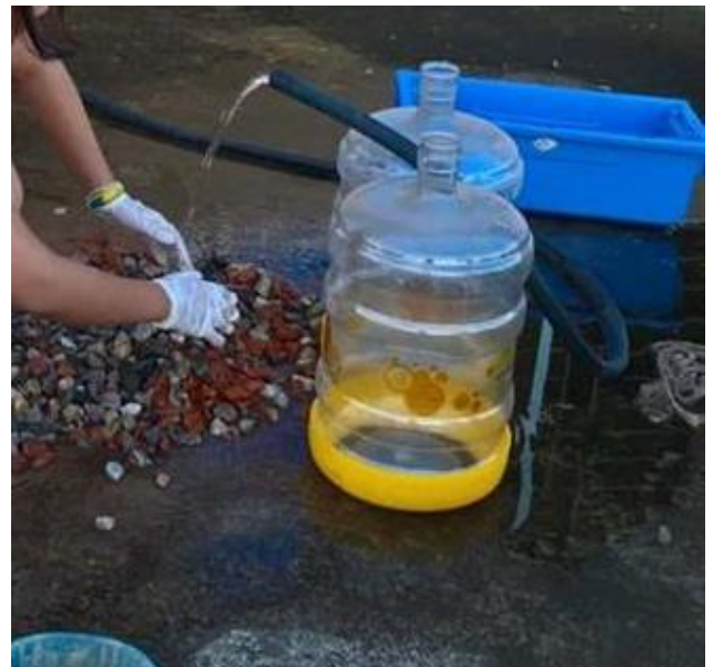
Figure 6: Brick Pieces Washing
