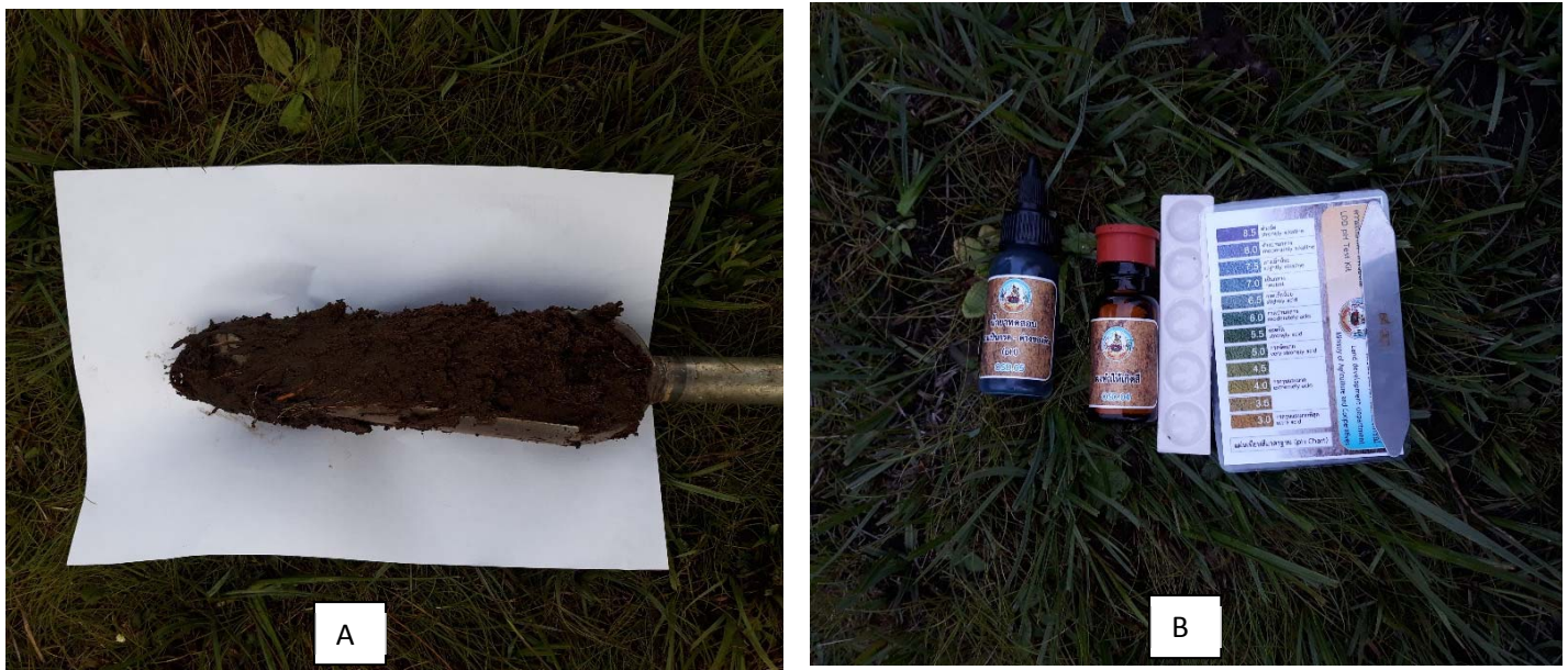
Figure 3. 4 (A): Soil sample collected at 20 cm depth using auger; (B): Field Soil pH testing kit
