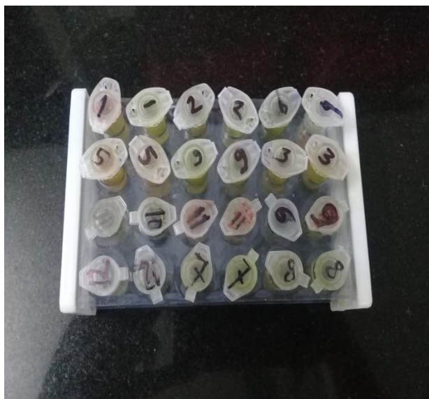
Image 4.1 : Eppendorf carrying acetone prior to centrifuging
